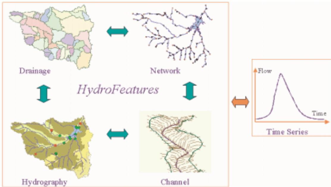
*Components of the Arc Hydro data model*
