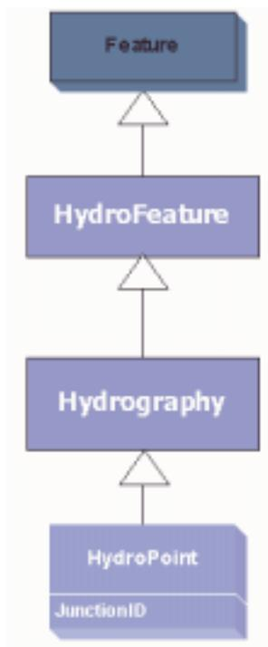
The *HydroPoint* class contains point features that are derived from map hydrography data layers.
