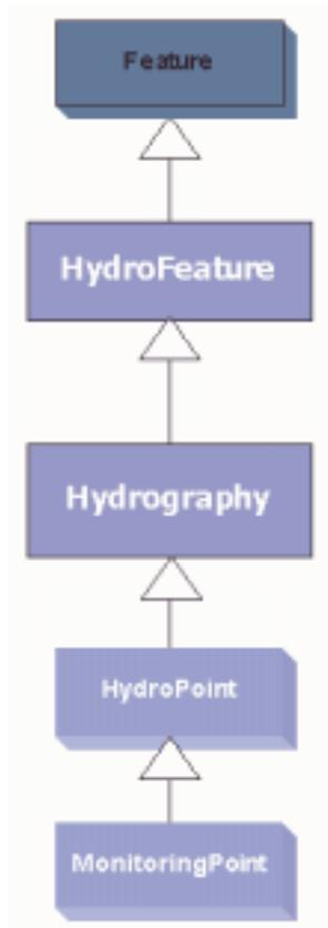
*Monitoring points* are intended to store the locations of gages that measure water quantity or quality, and may have time series data associated with them for analysis purposes. *Monitoring points* may also be subtyped or subclassed by the user. Examples of monitoring points include water quality monitoring stations, stream gage stations, rain gage stations, and any other type of fixed-location data collection points.
