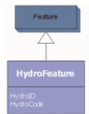
All simple feature classes in the Arc Hydro data model inherit from the *HydroFeature* abstract class.
