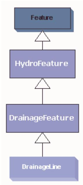
The *DrainageLine* is the line through the centers of the Digital Elevation Model (DEM) cells on a drainage path. It is produced when the DEM-based drainage paths are vectorized. *DrainagePoints* lie on *DrainageLines*. If necessary, the *DrainageLines* and *DrainagePoints* can be built into a geometric network and used as the Hydro Network for an Arc Hydro geodatabase.
