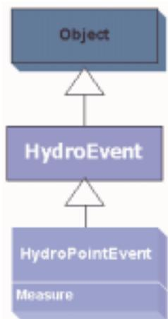
*HydroPointEvent* is a point event, which means a set of attributes attached to a single location on a line. *HydroPointEvents* can represent many things as the user can imagine in relation to natural water systems. Some examples are wastewater discharge points, USGS gage stations, and irrigation diversions.
