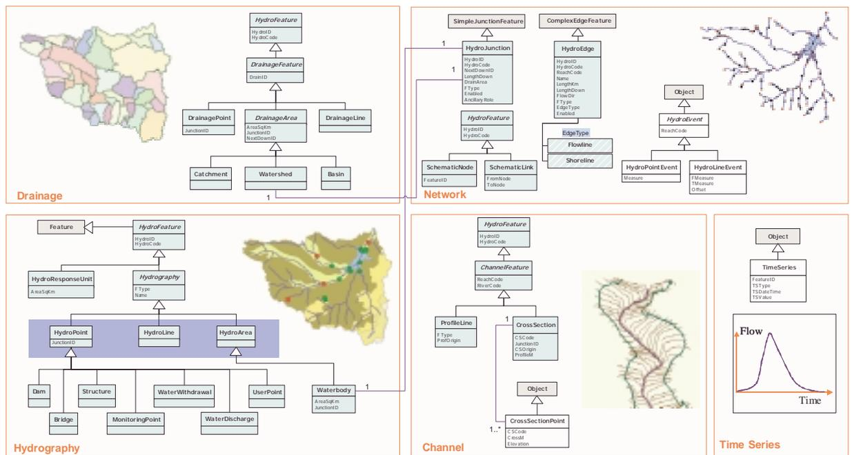
*Analysis Diagram of the Arc Hydro data model*
