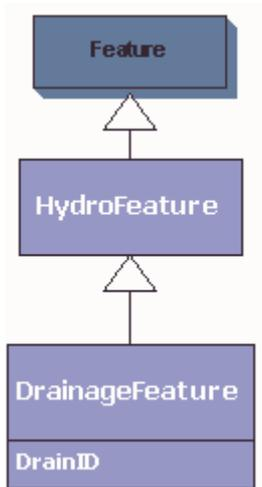
*DrainageFeature* is an abstract class, which inherits from *HydroFeature*
