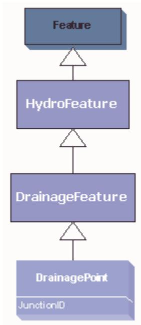
*DrainagePoint* is a subclass of *DrainageFeature*. A *DrainagePoint* represents the point at the center of a Digital Elevation Model cell at the most downstream location within a Drainage Area. The Drainage Area is associated with its Drainage Point using the *DrainID* attribute that both classes inherit from the *Drainage Feature* class. Drainage Points are also known as *Seed Points*, *Outlet Points*, or *Pour Points* of Drainage Area.
