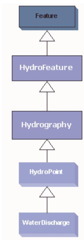
Water discharge points add flow to the stream network. Data on water discharge points is maintained by government agencies issuing permits for such discharges. Water can be discharged from wastewater treatment plants, by return flow from irrigation systems, or other sources. Typically, water discharges degrade the quality of the receiving waters, so these points are important for computing the water balance and water quality of natural water systems.
