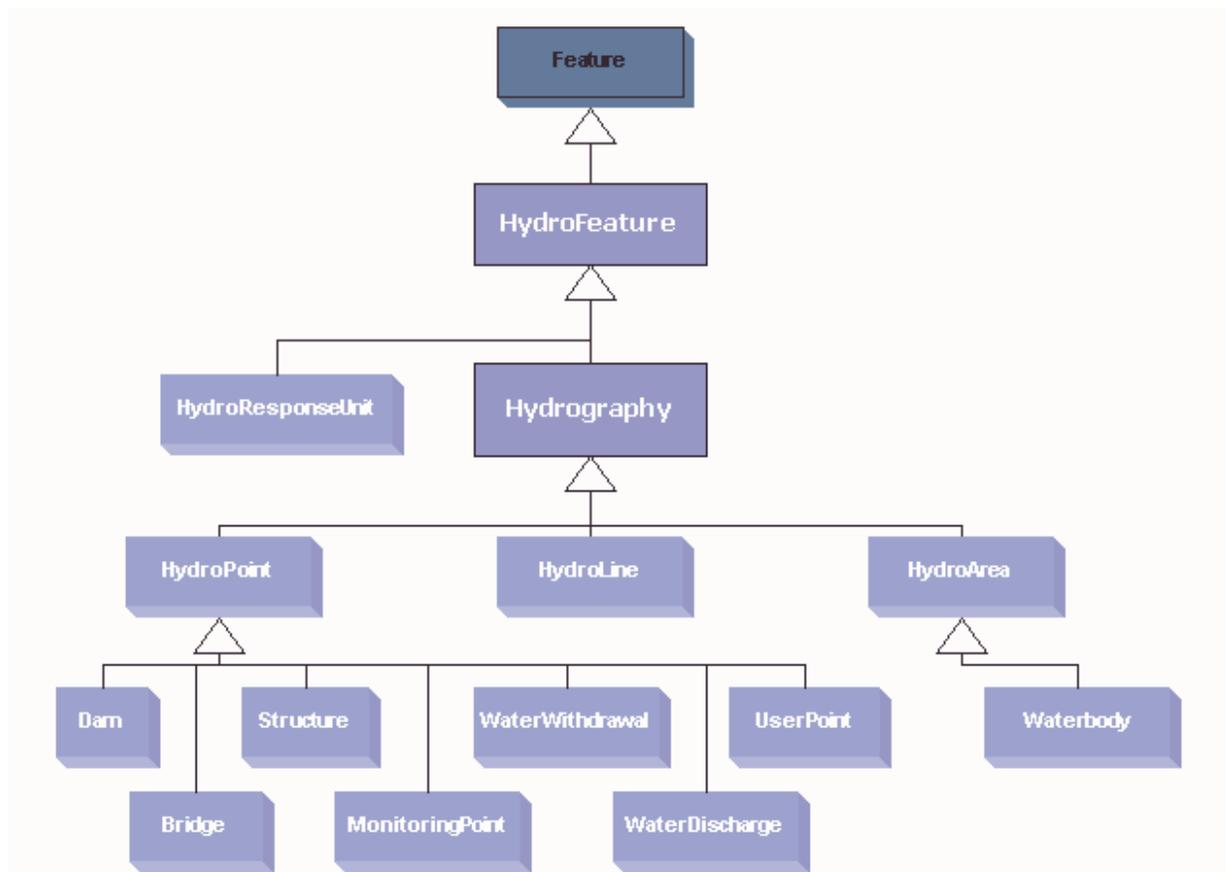
The *Hydrography* feature dataset contains the map representation of the surface water features. It contains several kinds of simple point, line and area features:
