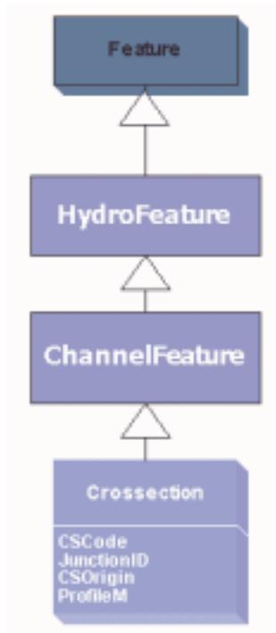
A *CrossSection* in ArcGIS is a 3-D PolylineM feature, where each vertex in the line is defined by four coordinates:  $x, y, z, m$ . The  $(x, y)$  coordinates give the location of the vertex in the horizontal plane,  $z$  represents the elevation above a vertical datum, and  $m$  is the CrossSection measure (*CrossM*), or distance along the CrossSection in the  $(x, y)$  plane.
