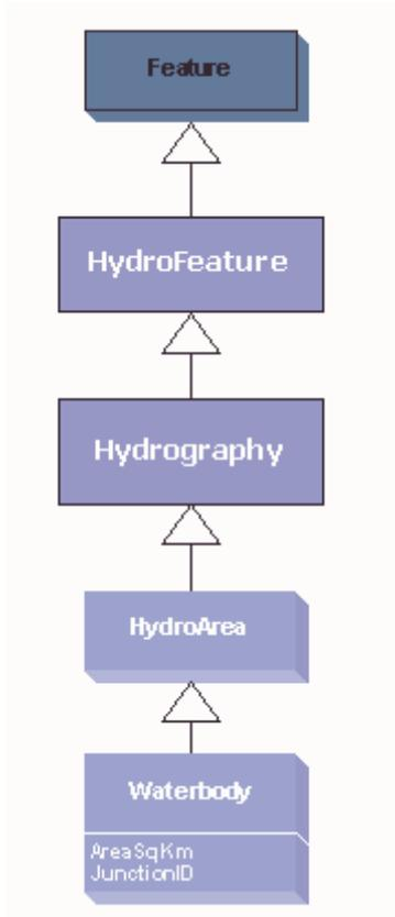
The *Waterbody* class is subclass of *HydroArea*, which represents water bodies such as lakes, bays and estuaries. The distinction between the *Waterbody* and *HydroArea* feature classes is that a waterbody may be a very complex spatial feature with many islands, and even component water bodies. The *Waterbody* feature class provides a generalized representation of waterbodies, for which additional detail is contained in the *HydroArea* class, if necessary.
