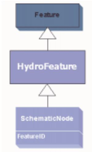
The *SchematicNode* feature class contains the points in a Schematic Network, which may represent any feature within an ArcHydro geodatabase. Typical types of SchematicNodes are: drainage area centroids, drainage area outlets, and stream confluences.
