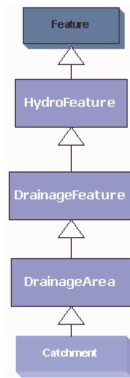
*Catchment* is a polygon subclass of *DrainageArea*. A *Catchment* feature class is an elementary drainage area produced by subdivision of the landscape using a consistent set of physical rules. Typically, this subdivision is carried out by defining a stream network from a threshold flow accumulation on a Digital Elevation Model, and then delineating a *Catchment* for each stream segment in the network.
