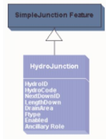
The *HydroJunction* class includes junctions between *HydroEdges* and other points that are vital to a network analysis, such as outlet points for drainage areas and locations of stream gages or other point features. *HydroJunctions* are points that stand for sources, sinks, stream junctions and other relevant user-defined locations. Among the *HydroJunctions*, sinks play a significant role in the analysis because each feature in the network drains to a single Sink.
