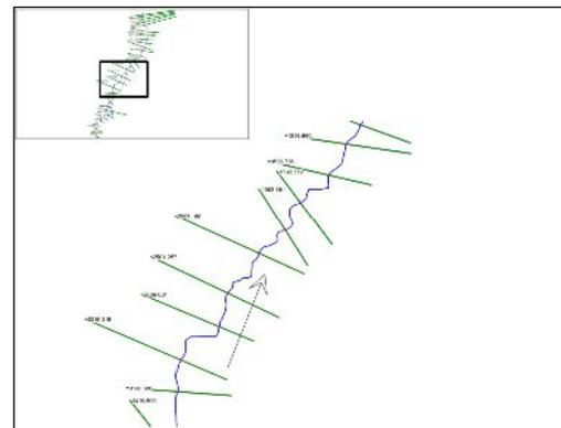
Figure 7. Geometric data generating from Hec-RAS.
