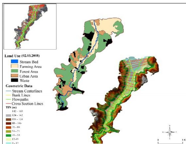
Figure 4. Using geometric data in flood mapping.
