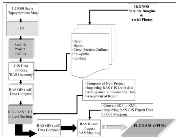
Figure 2. Flow chart of Hec-GEORAS and Hec-RAS Applications.
